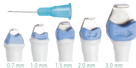
Ultrasonic sensing windows of Microvascular Flowprobe (MU) Series with a tip of a 25g. needle.
